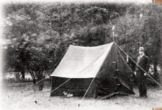
A photo from Mintrop's seismograph field manual shows the tent used to develop the seismogram after registration of the data. The tent has a red liner and constructed so that light cannot penetrate it.
