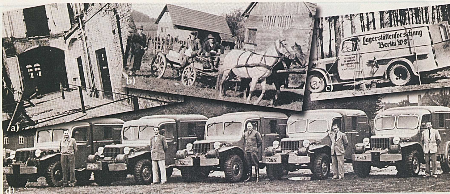
(a) Am Kleinen Felde 12—entrance to the first postwar Prakla headquarters in Hannover, 1947; (b) “shooting” truck in the Balkans—a wartime improvisation; (c) Phänomen Granit 25—first recording truck for reflection seismics; (d) old Dodge trucks of the U.S. Army were furnished with new cabins and equipped as seismic recording trucks.
