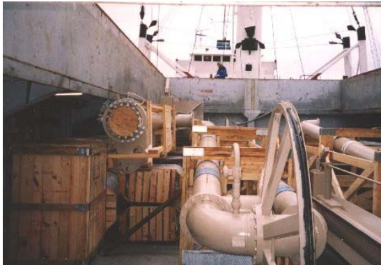
The crew did the lashing of the cargo. For the marine loading arms and the base risers the surveyor had recommended 5 lashings on each side.
